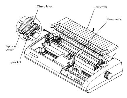
1 Remove the top and rear covers of the printer to insert the paper.
