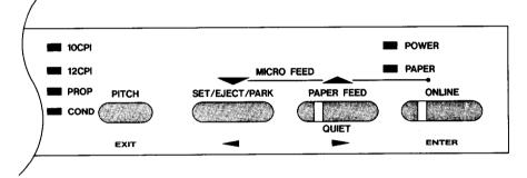
The principle involved is that the printer will print a list of options on one line. You use the settlectrane and (PAPER FEED) buttons to move the print head so that it is below the option you want to choose.
