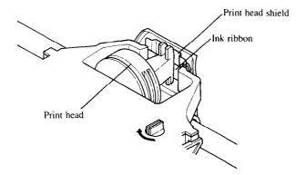
3 Use the grips on the side of the ribbon cartridge to help locate the cartridge (squeeze them inwards gently), and make sure that the spindles on the cartridge holder fit into the sockets on the cartridge itself.
